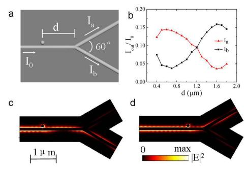
Figure 5 | Application of nanoparticle-mediated mode conversion for a tunable switch in a branched NW. (a) The sketch of the proposed switch structure. (b) The output intensities  $I_{out}$  at the two branches, normalized by the input intensity  $I_0$  as a function of particle locations. (c–d) Electric field distributions for the two states of power switched between the two output branches. The radiuses of the NW and the particle are both 60 nm and their separation is 5 nm.
